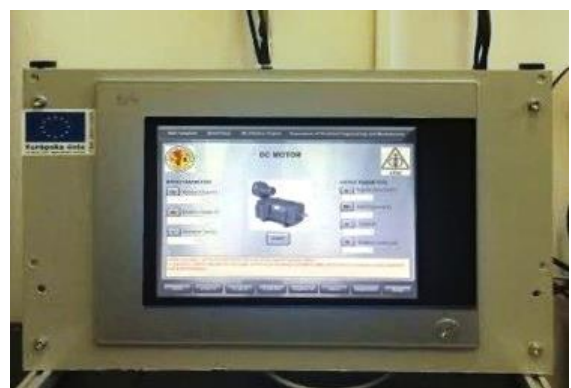
HIL working place for verification of control methods for drive systems
